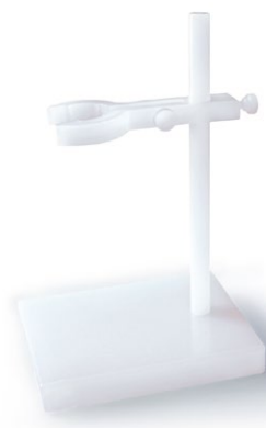
Bottle Stand PP. Full plastic construction. Support rod 325 mm, base plate 220 x 160 mm, weight 1130 g
