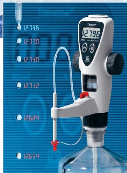
For titrations with visual detection of the endpoint, e.g., by changing color of the indicator or the formation of a precipitate, bottle-top or glass burettes are typically used.
