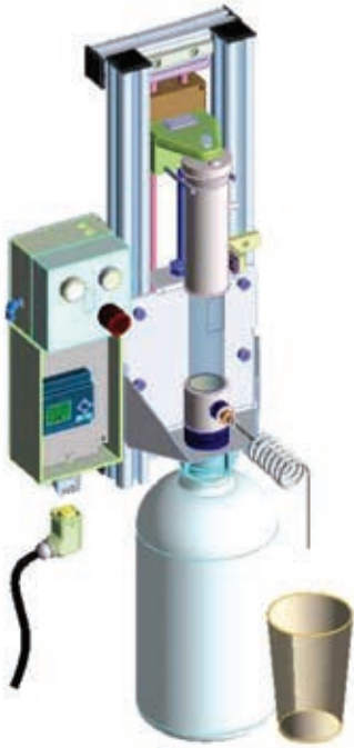
Pneumatic dispenser with PLC
