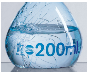
If the volumetric flask breaks, the shattering effect is reduced.
