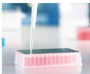
50 – 1000 µl pipette tips in a deep-well plate
