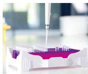
0.5 – 20 µl pipette tips in PCR tubes
