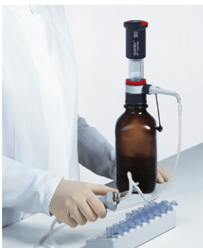
QuikSip™ aspirator with single channel device for removal of liquids out of reaction vessels, tubes, etc.
