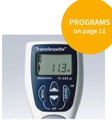
Pipetting with electrophoresis (GEL-mode). Program for loading electrophoresis gels.
