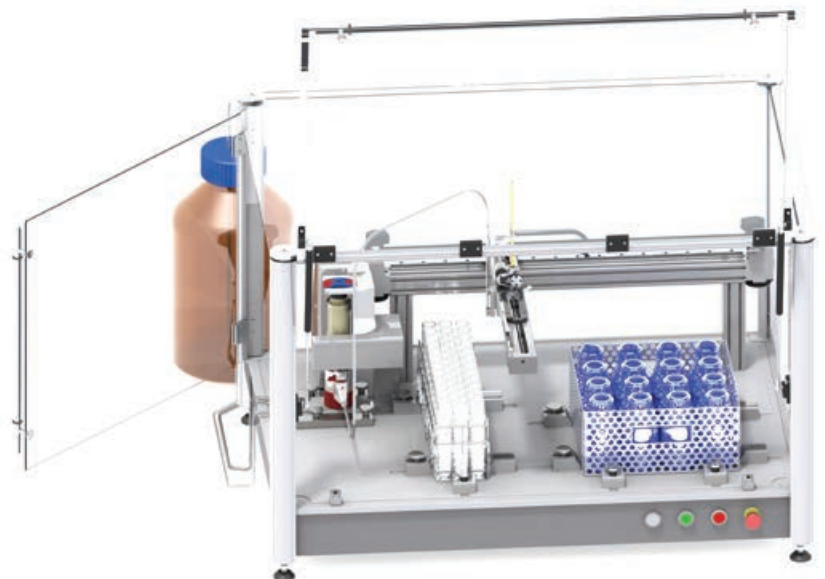
Single-channel Dispensing system with x/y/z portal
